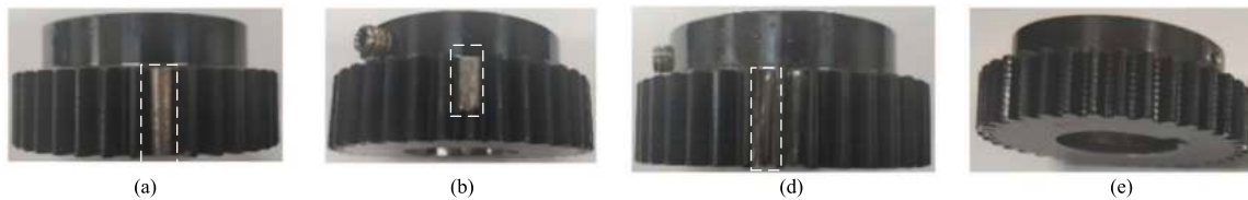
Fig. 7. (a) Miss (missing tooth), (b) Chipped (cracked teeth), (d) Root (crack at tooth root), (e) Eccentric (misaligned geometric and rotational centers).
